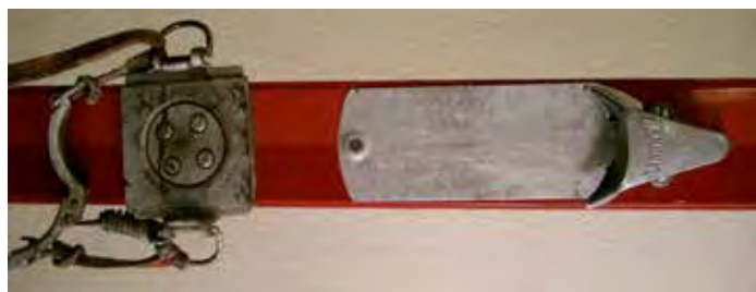
The Marker Simplex toe piece and turntable with longthong
